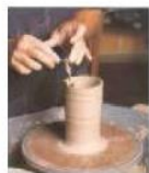
7 Any weaknesses around rims can be removed with a needle. With the wheelhead rotating slowly, steady the inside rim with the left index finger, and push the needle steadily into the clay wall approximately 1/4 in. (5 mm.) below the lowest point of the rim area. It needs your left index finger on the inside. Lift the cut section clear of the rim.
