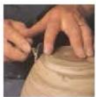
3 Taking up a comfortable position, join the fingers of both hands to form a steady line between hands, thumb, fore and pot. Steady by cutting away any unevenness from the base area and around the outer edge. If the outer edge is particularly ragged, it may be an advantage to use a needle.
