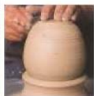
2 Chucks can be thrown especially for particular pots and then kept wrapped tightly in soft polyethylene until the next time they are required. Once positioned in the chuck, a turning can be done in the way described. If the pot is in the right state for turning, the clay will part off easily in long strips.
