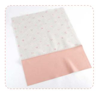
Sew a piece of faux leather to the bottom of each of the outer fabric pieces. Press the seam open and topstitch along each side of the seam. You will need to put a cloth over the seam when pressing so as not to melt the coating on the faux leather.
